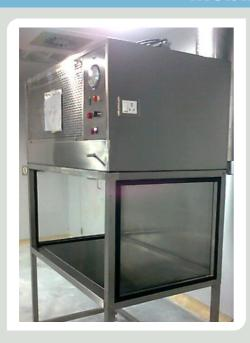
**Mobile Laminar Air Flow Unit** is designed for transporting sterile products under ISO Class 5 (Class 100) particle free work area to ensure product integrity. The work area is continuously supplied with positive pressure HEPA filtered recirculated horizontal / vertical air flow.
