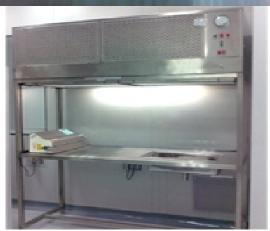
Vertical Laminar Air Flow unit is designed specifically for product protection. The Cabinet is a clean bench which provides ultra clean sterile HEPA filtered class 100 air in an isolated area for operations requiring a particulate-free environment where the highly sensitive process activities are carried-out.
