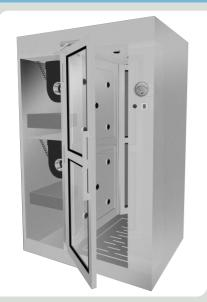
Air Shower is designed to supply Class 100 HEPA filtered air at high velocity it helps remove particulate matter from the personnel entering into the clean room. Air shower works as partial clean equipment installed at the partition between the clean room and non-clean rooms to shower the personnel or matters before entering the clean area. This unit helps to remove dust effectively and maintains the normal working status.
