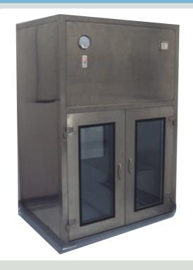
**Dynamic Pass Box** is designed to allow material transfer through controlled environment without much personnel movement to minimize man /material movement & avoid cross contamination between different classified areas. This is essentially installed to minimize movement of personnel for transfer of material into and from the clean room.
