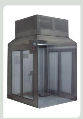
**Unidirectional Air Flow** Benches offers highest product protection for samples and processes by providing ISO Class 5 particle free work area. Unidirectional Air Flow unit draws air in through the top of the unit through a pre-filter, through a plenum and vertically down over the work-surface and past the lap of the operator. It has the advantage of not pushing air into the face of the operator as in a vertical laminar flow cabinet.
